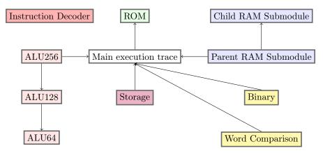
Figure 1: Modules of the zk-EVM. Arrows represent plookup inclusion proofs. N.B.: the Main execution trace, ALU, Storage, RAM, Binary and Word comparison modules also point to the instruction decoder.
