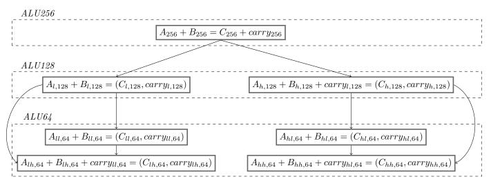
Figure 5: Field element decomposition and submodules communication inside the arithmetic module, addition example.
