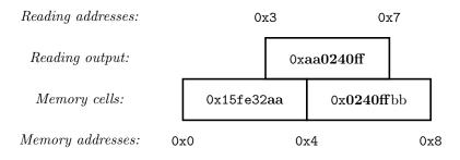
Figure 3: Overlapping reading process for words of 4 bytes.
