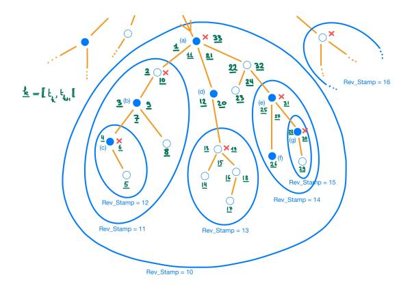
Figure 6: The above represents a portion of the tree of nested smart contract calls of a transaction. The solid blue dots represent calls to a given smart contract A, the hollow ones represent calls to other smart contracts. Red crosses represent reverts. The underlined integers  $\underline{k} = \llbracket t_k, t_{k+1} \rrbracket$  represent the *STORAGE\_TIMESTAMP* intervals wherein a given smart contract performs storage operations
