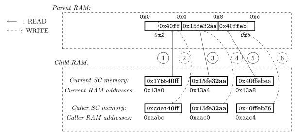
Figure 4: Illustration of the relations between the parent and the child RAM, for a RETURN instruction.
